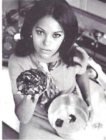
CLUSTER OF GARNET crystals, held here by Diane Johnathan of Bell Telephone Laboratories, was artificially grown in a solid platinum crucible like the one she also holds. Both the platinum crucible and the garnet are examples of increased use of precious metals and gemstones in Bell System research and development.
