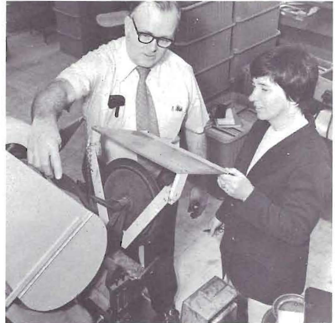
Safety Advisors Frank Curtin and Charmaine Doucet check the guards which O.S.H.A. requires on stamping machines.
