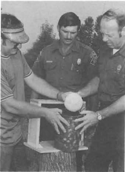
Barton and Conservation Officers Bruce Byrd and Jarret place an Audio Ball in a steel container. The steel is curved so that ricochets will not rebound towards the shooter, but be deflected towards the backstop.
