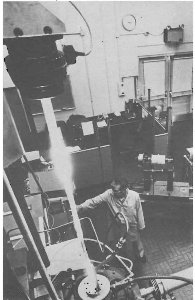
AT THE HELM - Western Electric technician Mike Hyle monitors a pilot production operation at the Atlanta Works, where precisely fabricated glass rods called "preforms" are softened (above) and pulled into hair-thin fiber lightguides. A cable containing twenty-four lightguides will be used in the Bell System's lightwave communications installation in Chicago.
