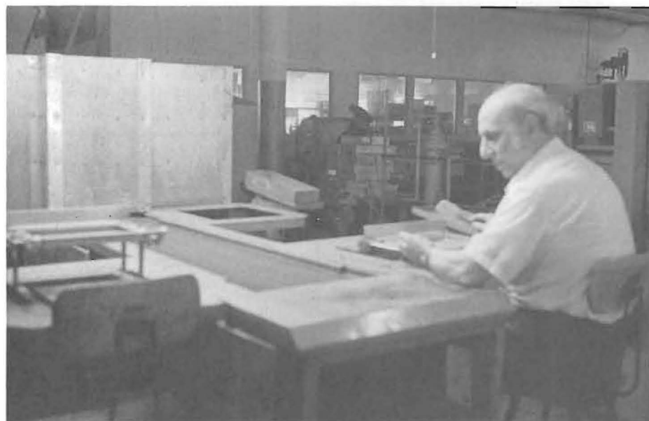
Tony Savinelli sits at the screening oven in Lawrence where for 26 years he placed mica strips to be silver laminated for mica capacitors.
