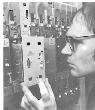
Helping computers talk to each other will soon be the job of this Western Electric dataport being slipped into place in a test model of a telephone voice-channel bank by Senior Engineer John Schaefer.
