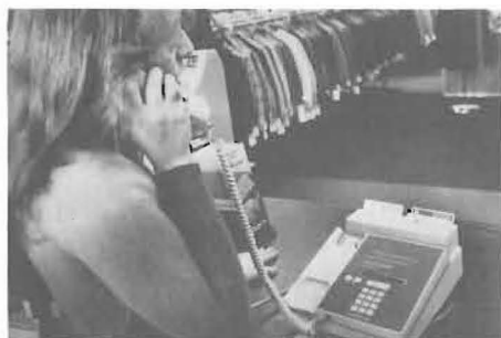
CREDIT CHECK - Ann Jyacek of clothing store in Long Island, N.Y., checks a customer's credit over Transaction II, Western Electric's telephone/data terminal. Transaction II is connected directly to a credit authorization center's computer for fast verification.
