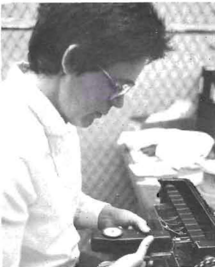
Dianne Weeks administers pull test to solderless wrapped connection.
