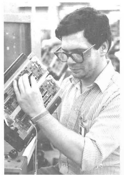
Jeff Page, utility operator in the D5 Assembly and Mass Solder Dept. at Merrimack Valley Works, does hand-insertion on an AEK21 channel unit which is sensitive to static electricity. He wears a special electrostatic discharge (ESD) strap, which is grounded, on his left wrist.
