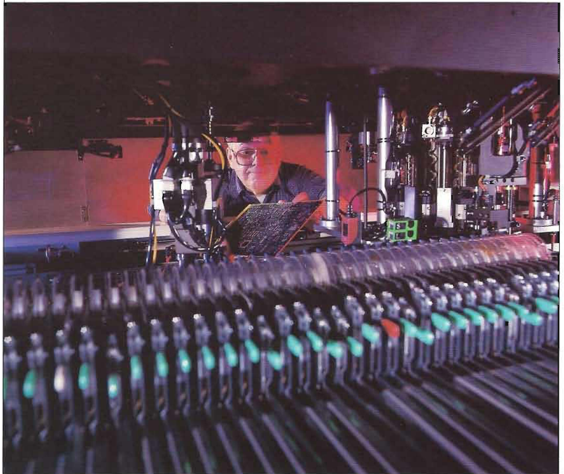
Dick Leduc, machine setter, inspects the setup of the Panasonic high-speed pick & place machine in the VISION surface mount area.
