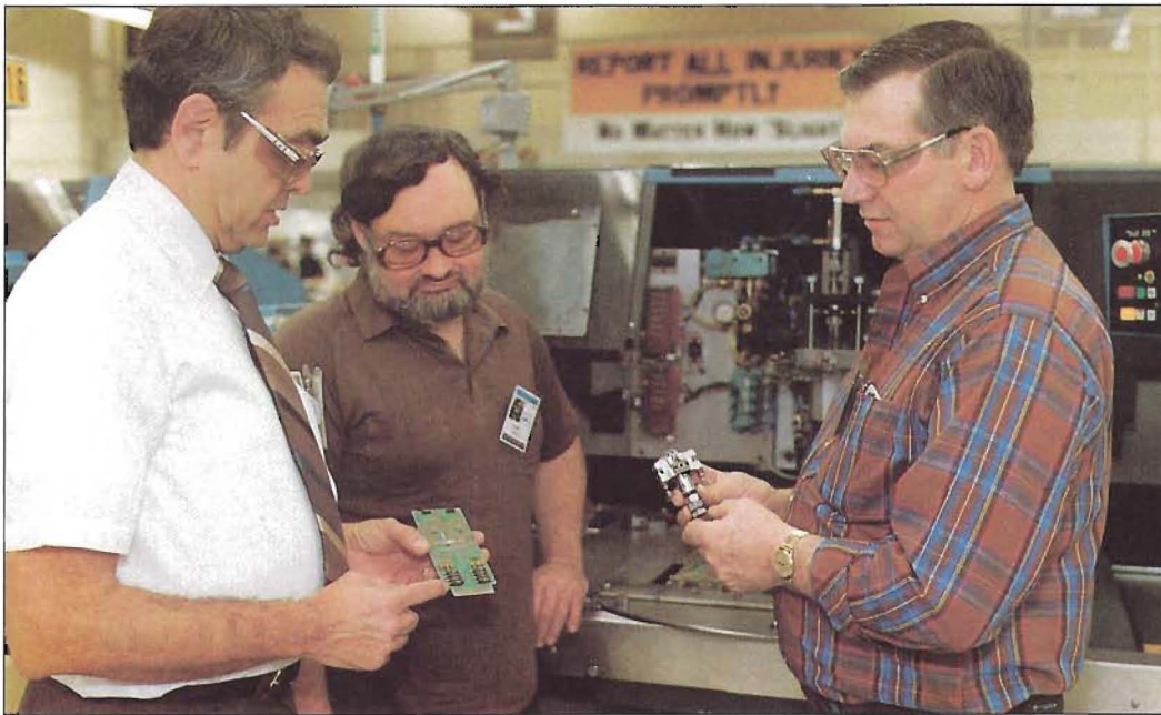
Machine System Technicians Bill Welch and Glenn Smith suggested switching to carbide cutters in the radial insertion machines used in the Patriot shop. In this photo, from left, engineer Jim Connors, Glenn and Bill discuss some of the benefits of the new cutters.
