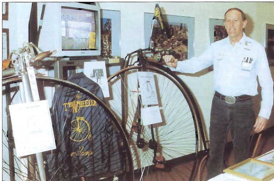
Bob Hartson, a member of the NH Wheelmen, explains that style was not the reason for large front wheel. Before chain drives were added to bicycles, the larger wheel allowed more distance per revolution, thus easier pedaling through the muddy streets of the 1880s.
